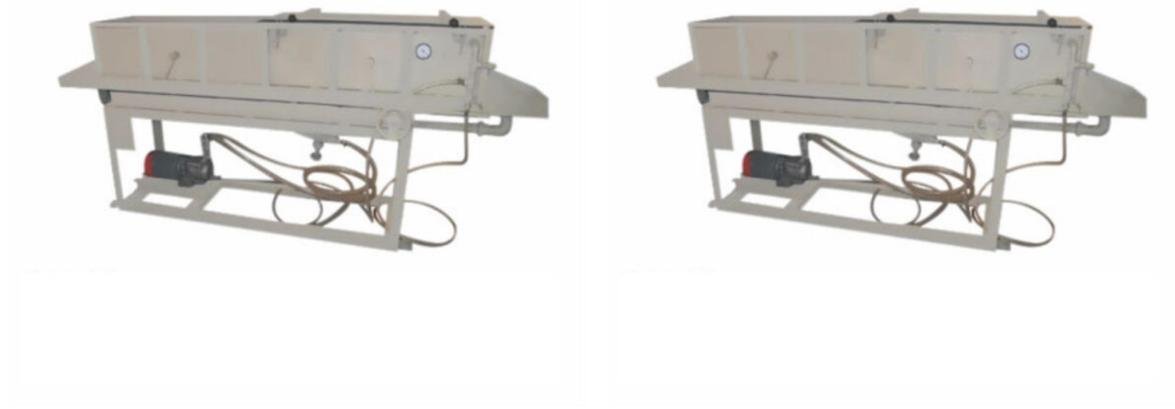
Water tank with sprays and without sprays for cooling of the pipe.
